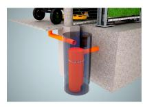
I) Copper filter placed in front of the reservoir of a VG Biobed <sup>tm</sup>
